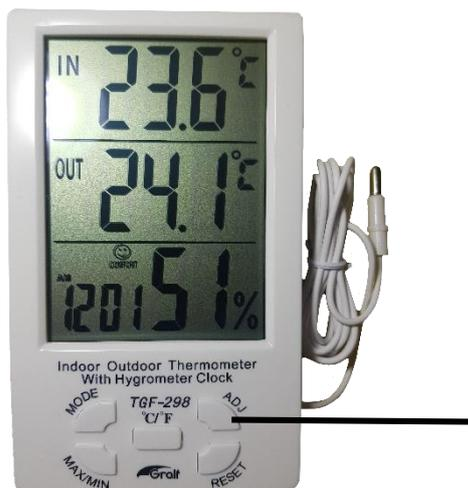
**EN MODO DE AJUSTE DE HORA: SOLO INCREMENTA EL TIEMPO, PRESIONELO HASTA LLEGAR A LA HORA DESEADA**
